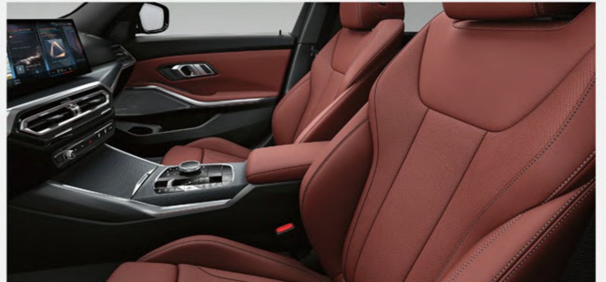
Sport seats for driver and front passenger in perforated Sensatec can be adjusted electrically, including memory function.
